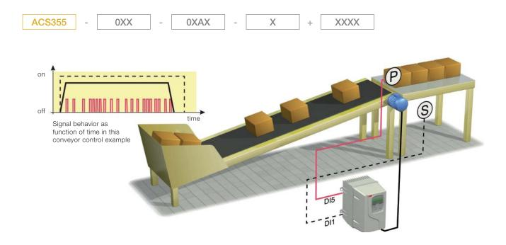
The ACS355 drives have many solutions for common challenges. The following example explains how the COUNTER STOP function operates within a conveyor unloading routine. The function stops the conveyor after a predefined number of boxes have passed the sensor.
