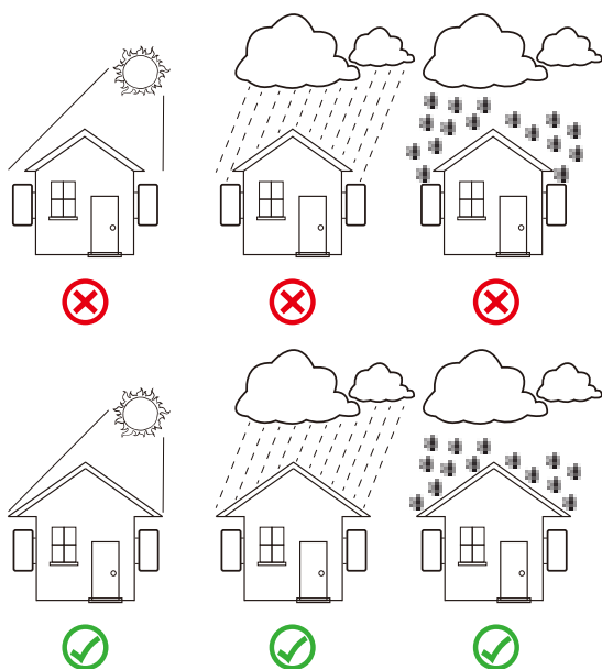
Pic 4.1 Recommended installation place
