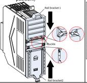
vertically on the DIN rail, and push sheet metal lock catch upwards to make it tightly engage with the rail.
