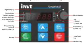
Figure 5-1 Standard LED keypad
