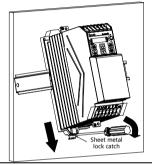
the DIN rail bracket inward, and then pull out rail brackets 1 and 2.
