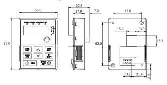
Figure D-5 Keypad openings without a bracket
