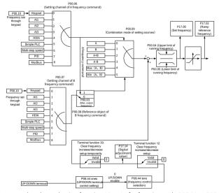
For example, when selecting function 10 or 11 for function code P05.01 or P05.02, S1 or S2 is the Up or Down terminal. When S1 or S2 is closed, the reference frequency
