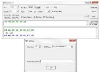
Set Port to COM1. Set BaudRate consistently with P14.01. DataBits, Parity, and StopBits must be set consistently with P14.02. If the RTU mode is selected, choose Input HEX and Show HEX. To implement automatic CRC, you need to choose ModbusRTU, and set Start Byte to 1 and CRC Type to CRC16 (MODBU SRTU) in the CRC Settings window. After the automatic CRC is enabled, do not enter CRC in
