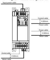
Figure 4-4 Cable routing distance
